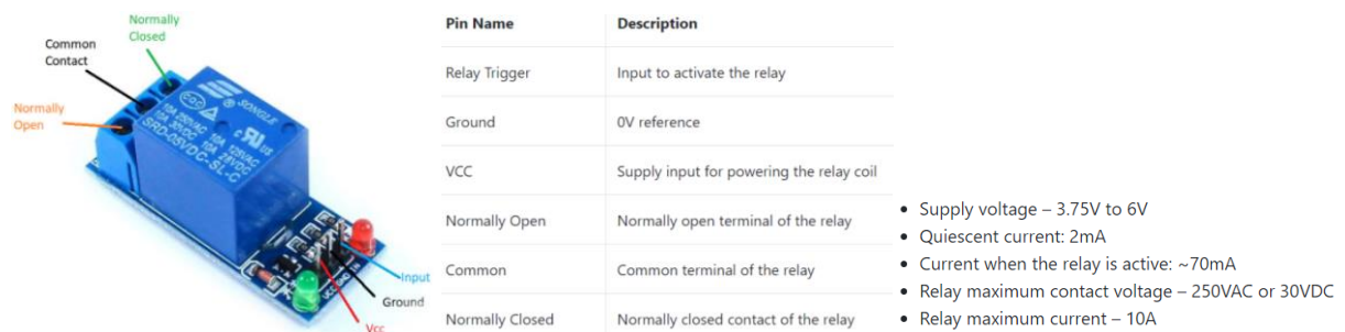
Figure 2.45: Relay module pinout diagram, description and specifications [81].
