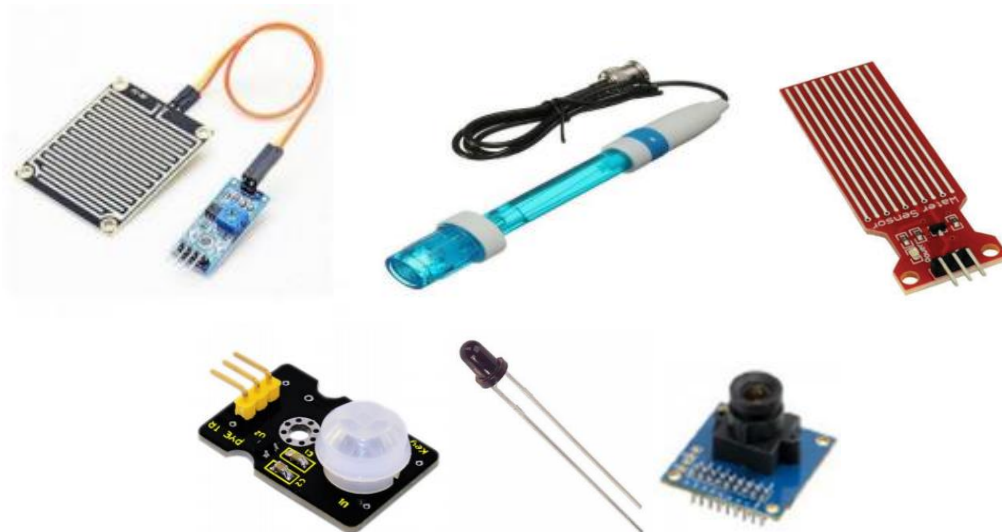
Figure 1.25: (a) Rainfall detection sensor [39], (b) soil pH sensor [38], (c) water level sensor [1], (d) PIR movement sensor, (e) HPTB3b-14D fire sensor [42], (f) VGA camera OV7670 module [43].
