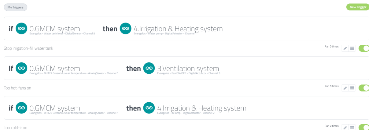
Figure 3.21: Automatic greenhouse micro-climate control with Cayenne triggered actions.
