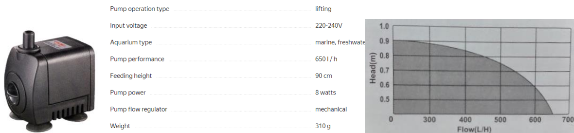
Figure 2.44: Submersible water pump XiLong XL-780 specifications and head-flow diagram.
