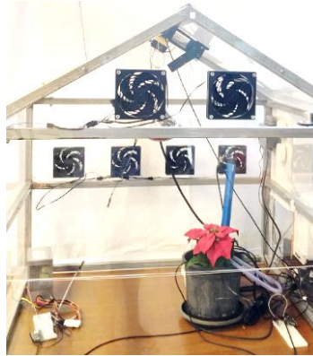
Figure 3.14: The implementation of the dynamic ventilation system.
