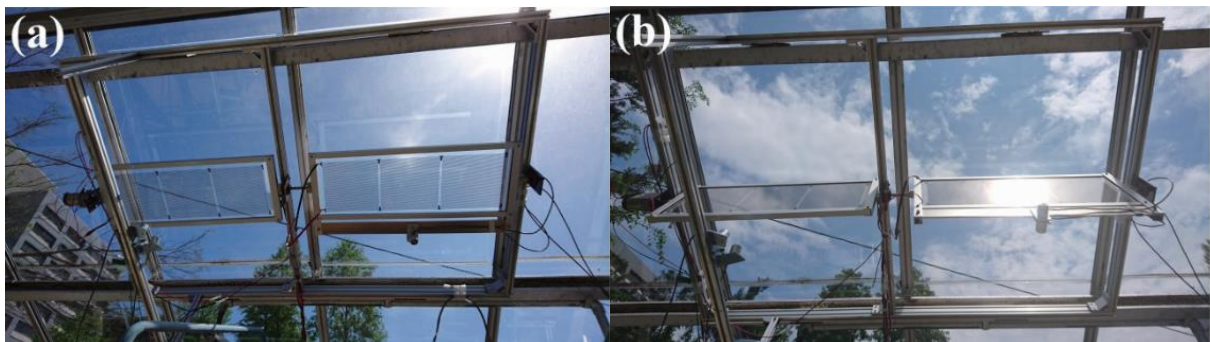
Figure 1.11: Semi-transparent PV modules positioned parallel (a) or perpendicular (b) to the roof surface [23].
