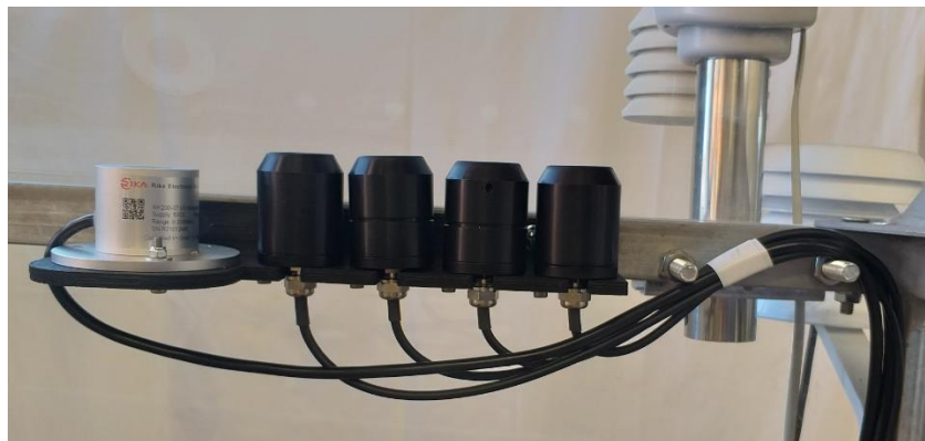
Figure 3.6: 3D printed sensors holder.
