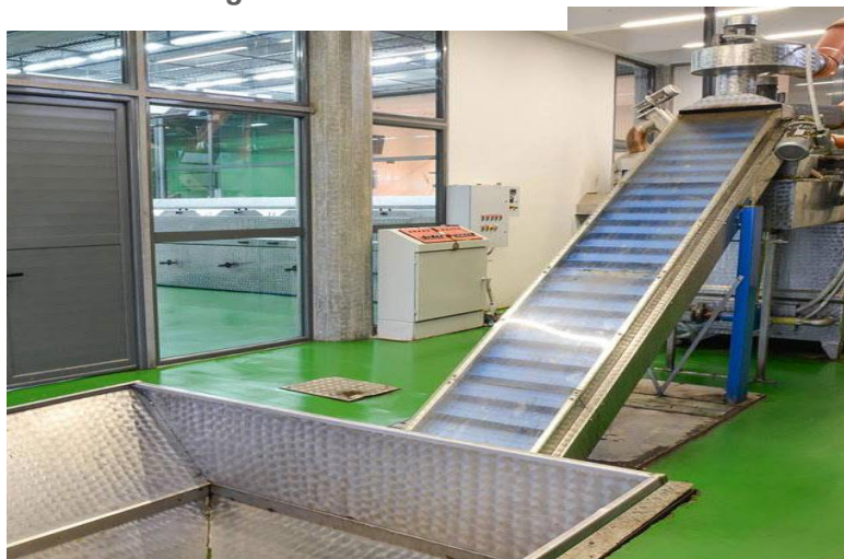
Figure 11. Convey belt with de-leafing
