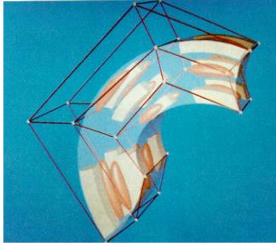
Figure 2.1.24 The modified lattice containing the deformed object (Sederberg and Parry, 1986).
