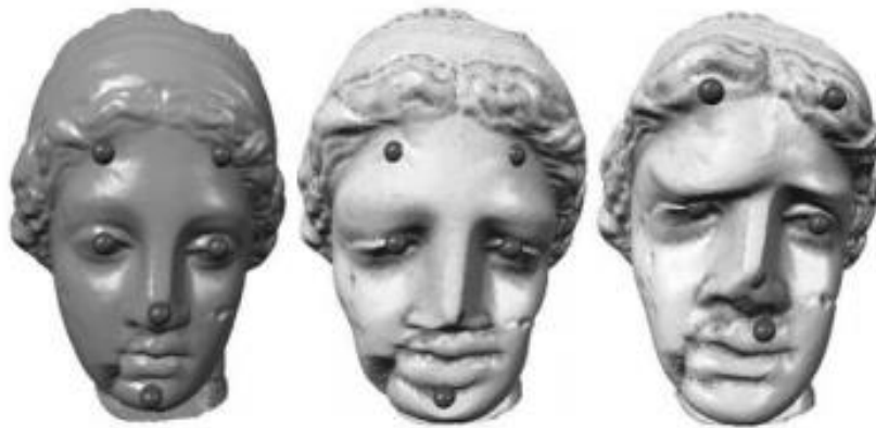
Figure 2.1.9 Left: The input geometry and six control points placed on it. Middle and Right: A sequence of deformations produced by the alteration of control points' position (Yoshizawa et al., 2002).
