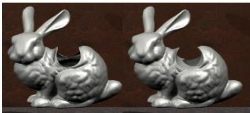
Figure 2.1.14 Left: The Stanford bunny model cut with a cylinder tool from above. Right: The DFFD's stitching algorithm was applied in order to close the opening (Schein and Elber, 2004).
