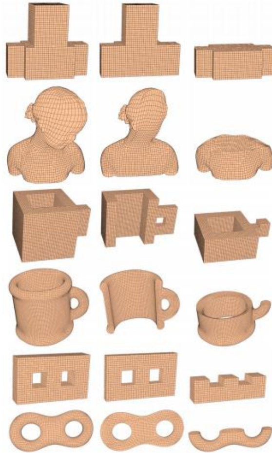
Figure 1.6.20 The generated hexahedral mesh using the Direct Product Volumetric Parameterization method (Xia et al., 2010).
