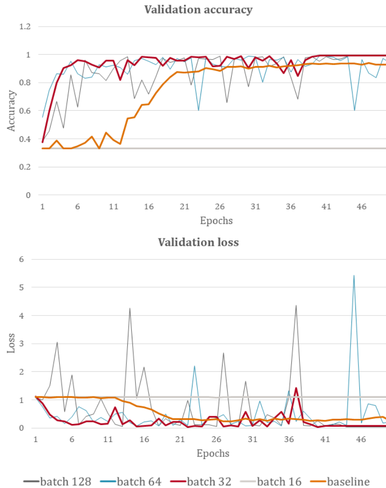
Figure 6.25: Comparative charts showing the resulting learning curves for each batch size tested using Adam optimizer with a learning rate of 0.001 on dataset-B. The baseline learning curves are presented for comparison reasons. Batch 32 is selected as the training setup for Model 2.
