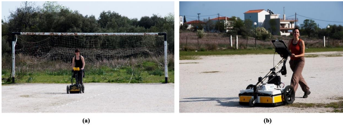
Figure 3.8: GPR survey at Demetria's soccer field. (a) Single-channel Noggin GPR equipped with a 250MHz antenna operated by Merope Manataki and (b) the multichannel Mala Mira GPR equipped with 400MHz antennas operated by Dr. Carmen Cuenca-Garcia.
