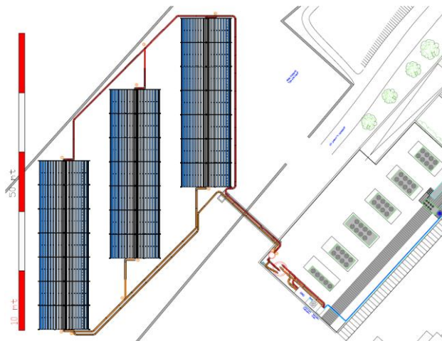
Figure 38: General plan of the solar field in Palermo with three parallel rows of linear fresnel collectors [215]
