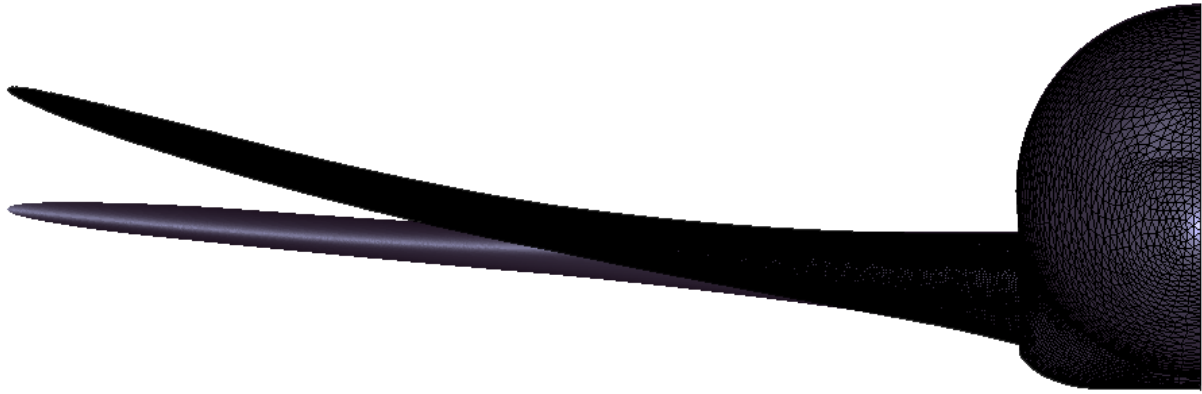
FIGURE 5.7: Parabolic deformation of the NASA CRM aircraft wing (max deflection 5 m at wing tip).
