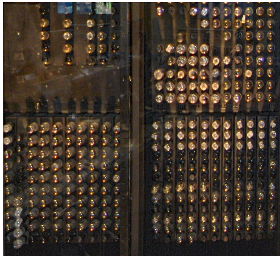
FIGURE 2.1: Detail of the back of a section of ENIAC, showing vacuum tubes: URL
