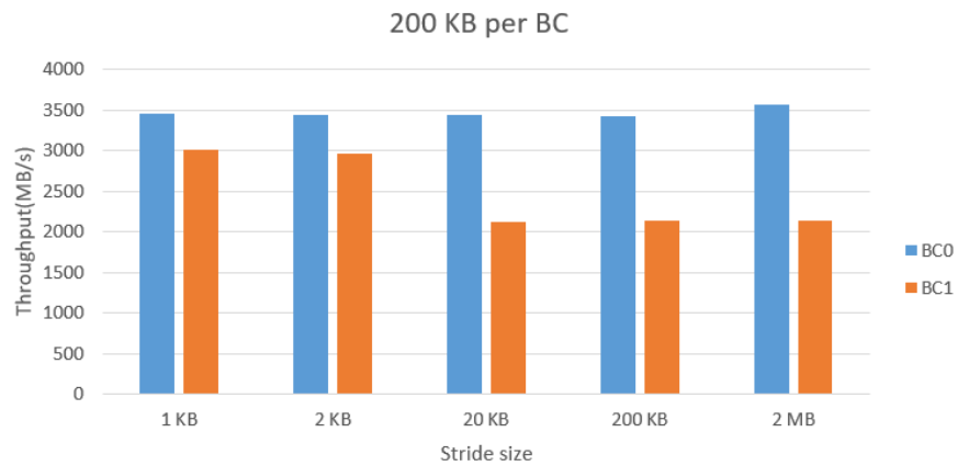
FIGURE 6.9: Results for different memory strides when each BC requested 200 KB.
