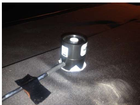
Image 3. Left: One of the illuminance sensors. Right: The data logger.
