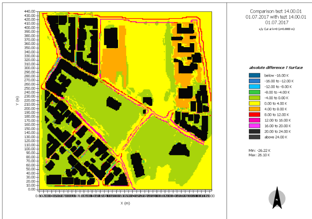
Figure 36: Comparison Cool and Green Pavement Scenario - Baseline Scenario Surface Temperature (Time 14:00).
