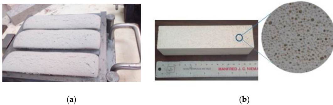
Figure 6. (a) Mixtures cast into 40 \times 40 \times 160 \text{ mm}^3 molds after aeration; (b) specimen with flattened surface.
