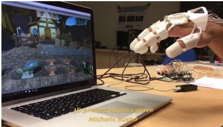
Figure 15: A Haptic Glove Prototype for Tactile Feedback in 3D Interactive Applications
