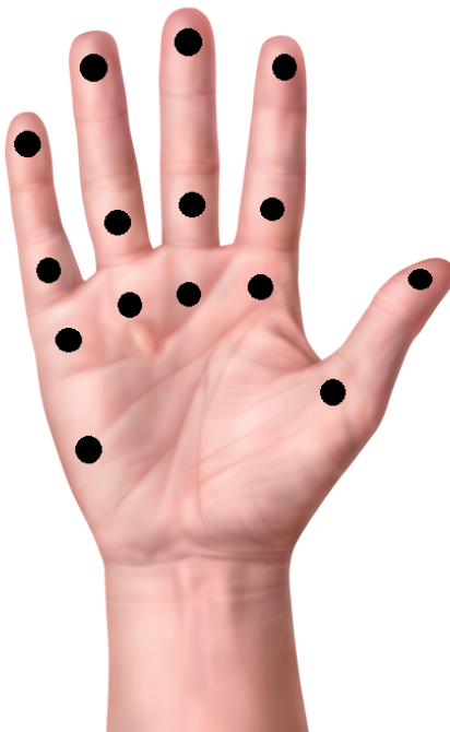
Figure 1: Position of vibration motors on the hand
