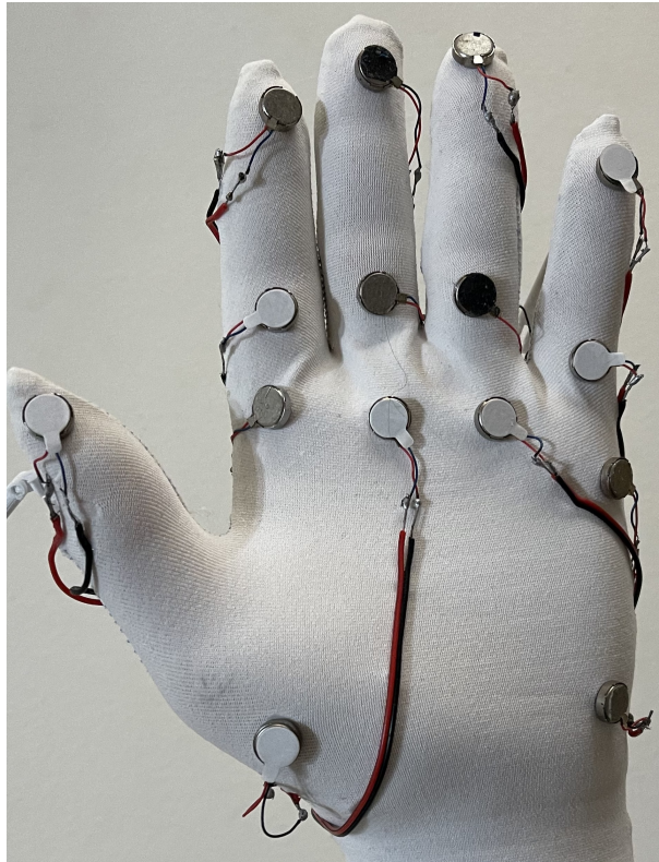
Figure 3: Bottom view of the haptic device
