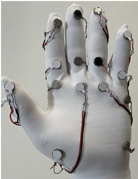
Figure 18: Bottom view of the haptic device
