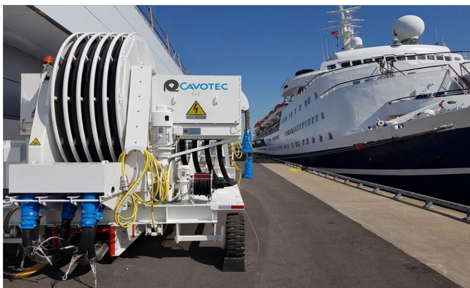
Figure 2.10 AMP Mobile Truck of CAVOTEC [7]
