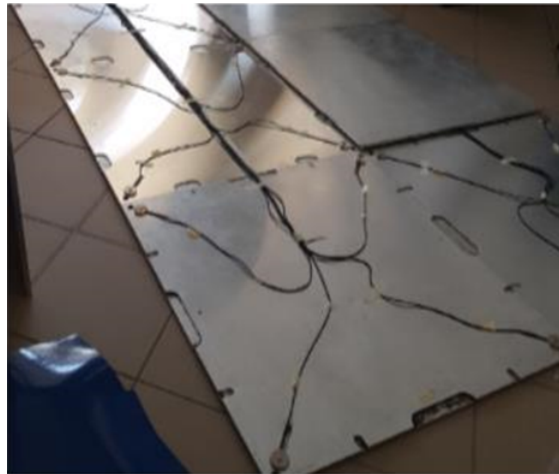
FIGURE 5.2: Force sensors installed beneath the vertices of the plates. [17, 39]
