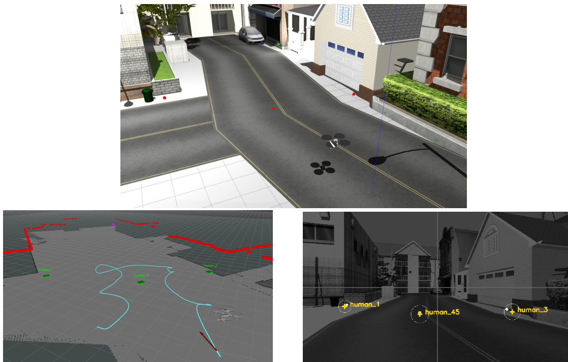
Figure 4.43: Targets localization by the UAV and their illustration in the rescuing map. The green markers depict the approximated positions of mapped targets. As the targets have been positioned, they are viewable within the image frame of the UAV’s cameras.
