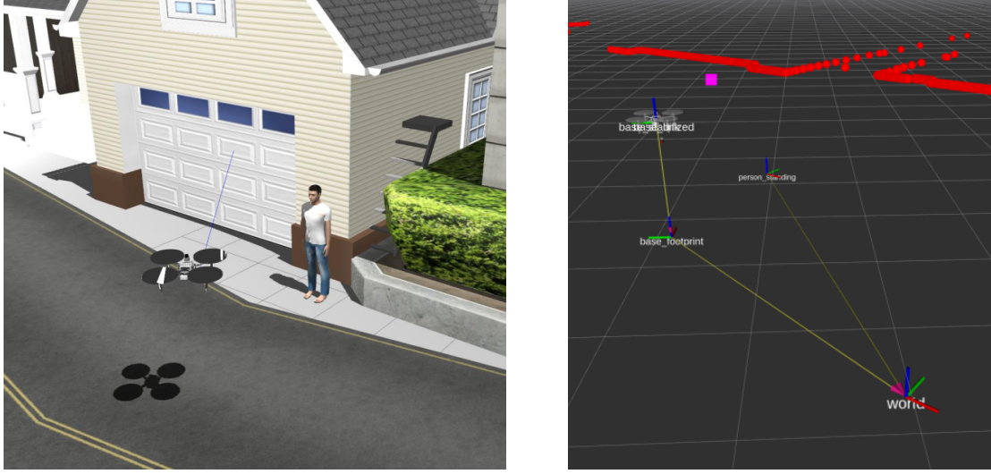
Figure 4.23: Gazebo environment and the corresponding coordinate system relations.
