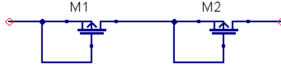
Figure 6.7 Diode-connected transistors in series acting as a high resistor
