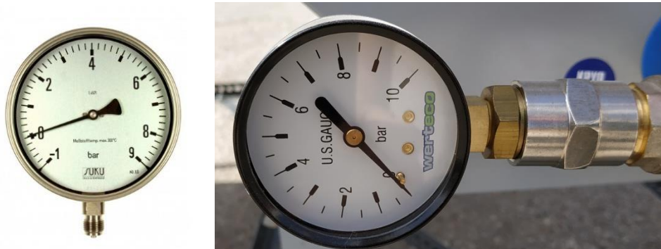
Figure 2.61: Standard Bourdon tube pressure gauge
