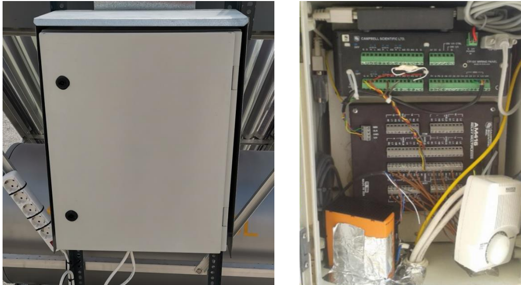
Figure 2.41: The data logger, the thermocouples, the power supply of the flowmeter and the dimmer
