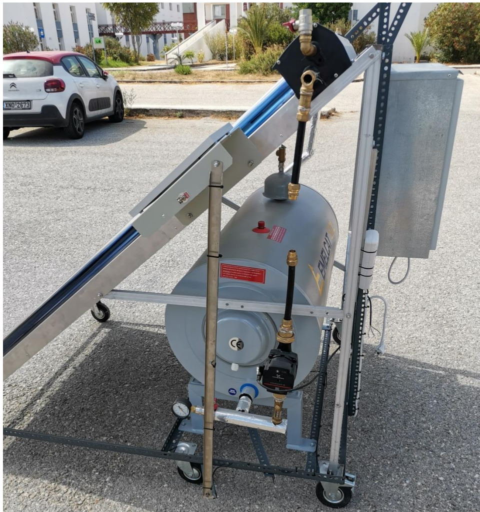
Figure 2.38: Creation of a closed circuit with the installation of a circulator and a flowmeter
