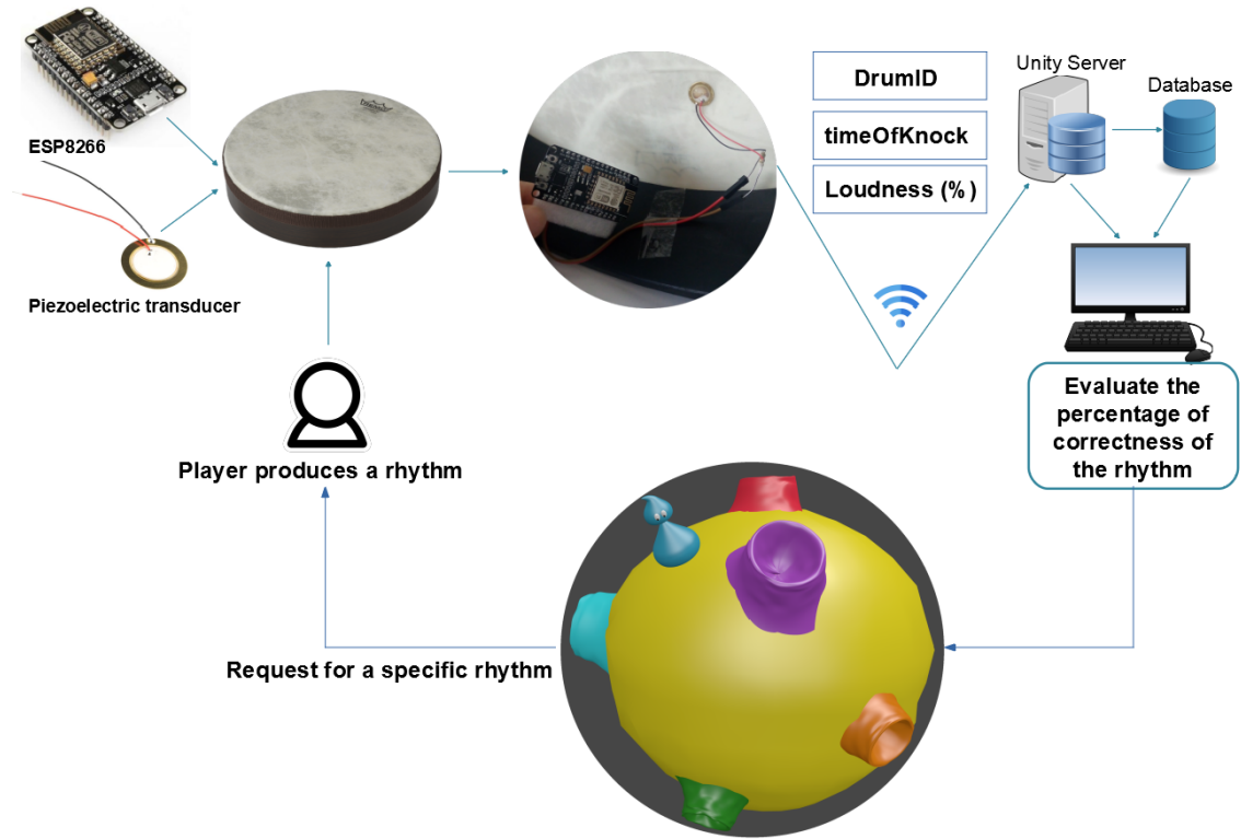
Figure 7: Architecture of the game using ESP8266 & sensor
