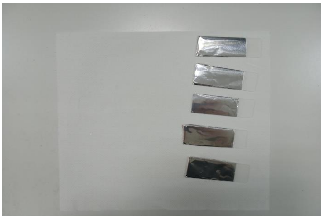
Lab Photo 18: We put aluminum foil on top of microbiological glasses
