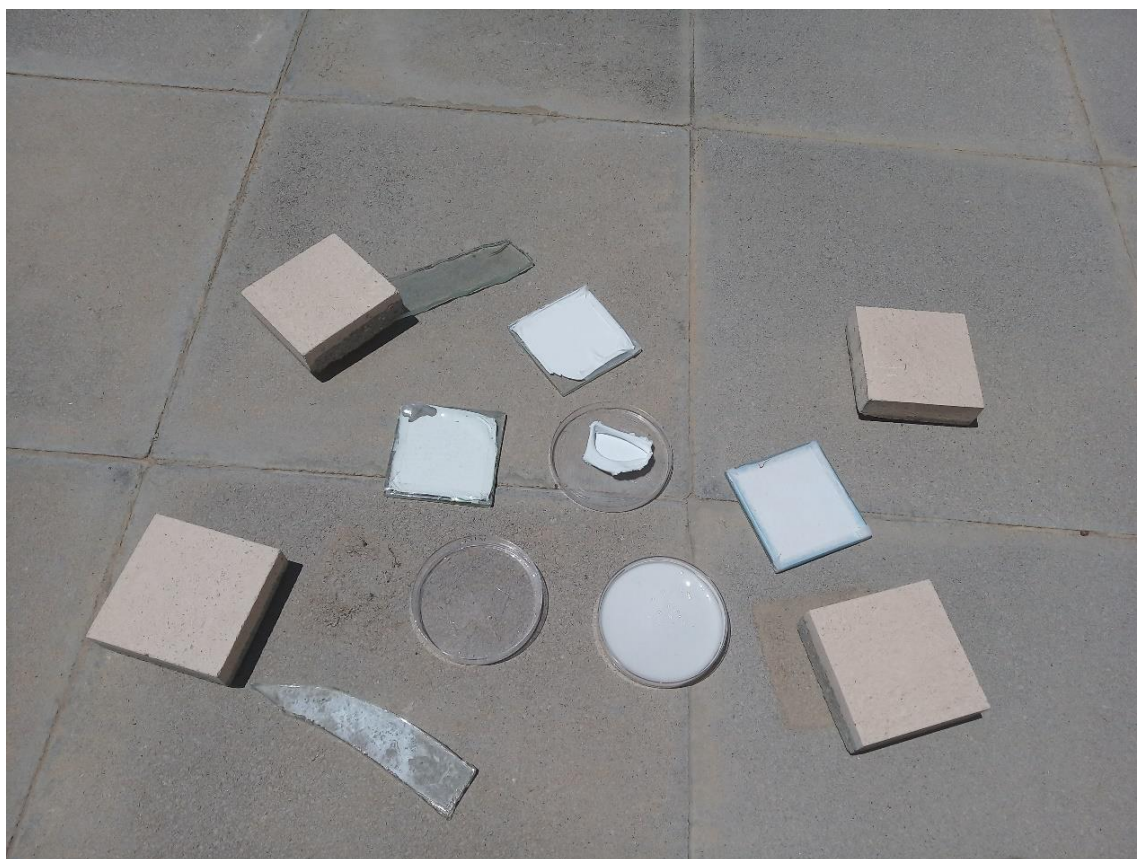
Lab Photo 36: Placing the samples on the rooftop in order to be measured with a thermal camera. From top to bottom and from left to right: porous polymer (no dye), green porous polymer, blue porous polymer (#2), blue porous polymer, waterglass and \text{NaZnPO}_4 (thick) surface (#2)
