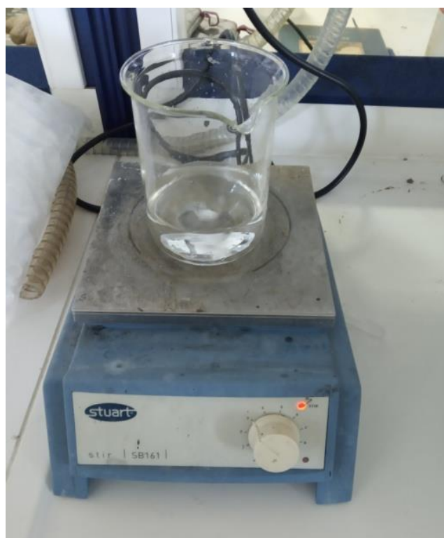
Lab Photo 11: Stirring the solution after adding the \text{H}_3\text{PO}_4
