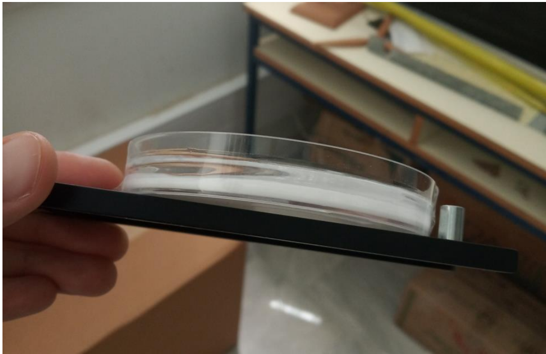
Lab Photo 35: Preparing the \text{NaZnPO}_4 sample (#2) to be measured by the spectrophotometer.
