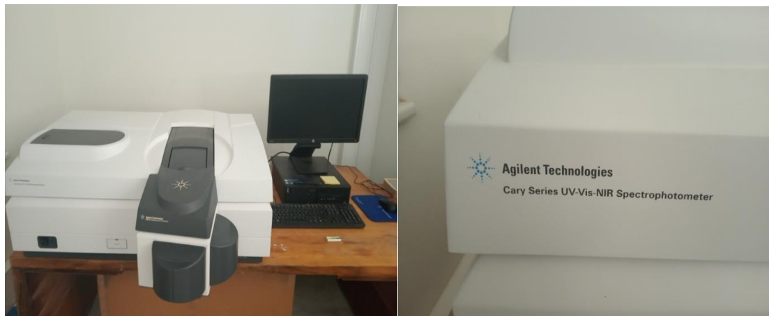
Lab Photos 37 & 38: UV – Visible – Near – Infrared Spectrophotometer and the associated computing system
