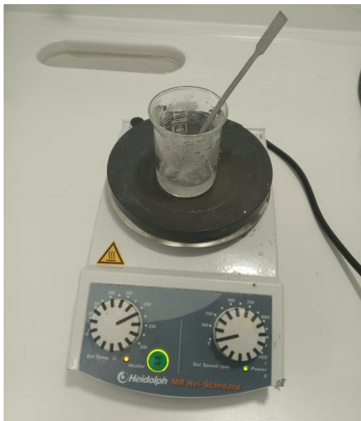
Lab Photo 24: Heating and stirring of waterglass
