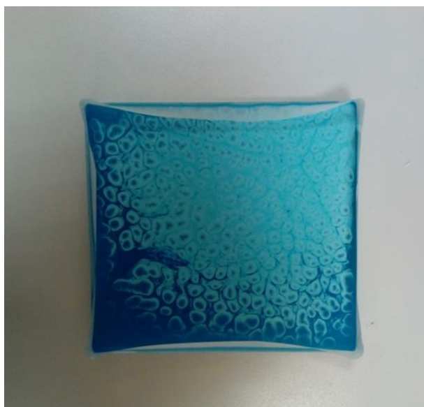
Lab Photo 6: The second blue color batch where we added 1 ml of food blue color. After the first few hours the dye seemed to be staying at the bottom, so the front surface developed a lighter shade of blue color than the back side.
