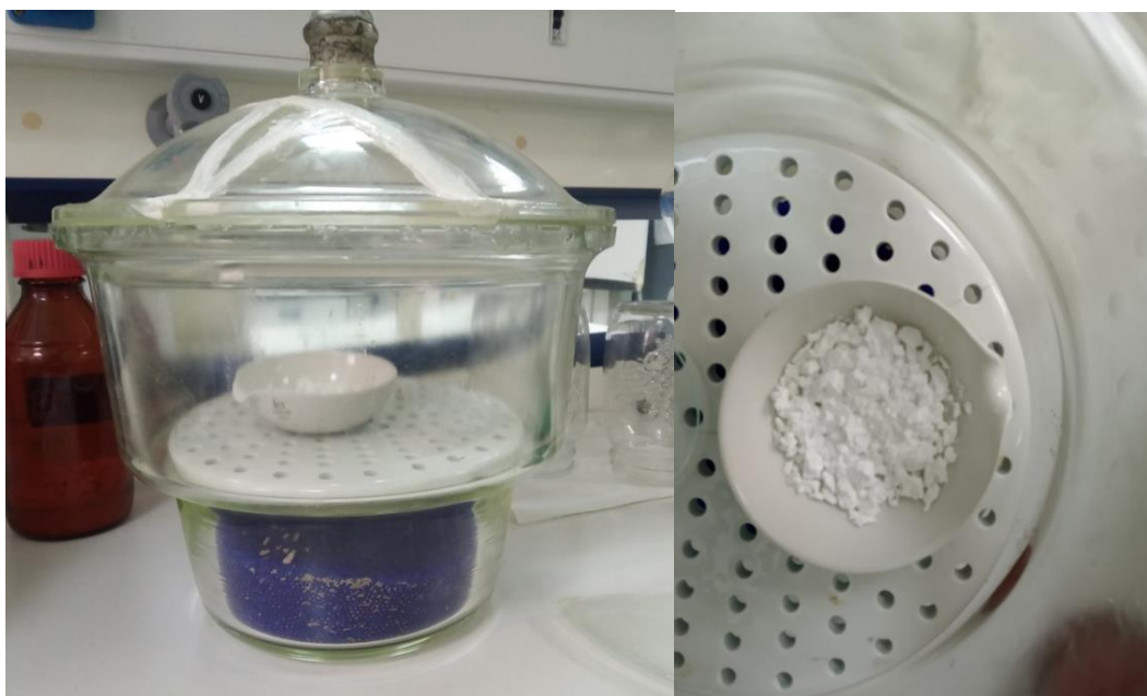
Lab Photos 14 & 15: We leave the powder to cool at room temperature
