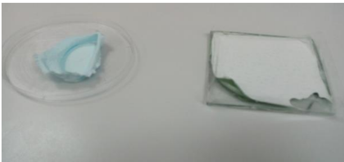
Lab Photo 5: The first batches. On the left we can see the sample with 0,8 ml of blue food color put on a PET basis while on the right we can see the green mineral color sample which was placed on a glass carrier.
