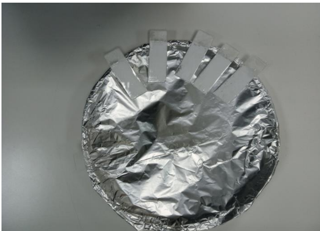
Lab Photo 19: We created the surface by spraying the solution on the aluminum foil
