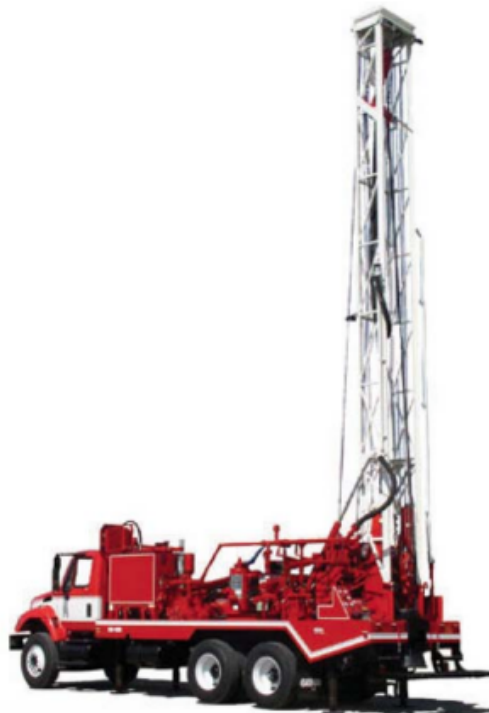
Figure 1.6: Rig with cantilever derrick (Derrick Engineering Company 2010) and Mobile rig with portable mast (GEFCO 2007), Courtesy of GEFCO .Figure retrieved from [23]).
