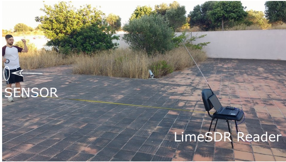
Figure 4.2: Ambient reader experimental setup.
