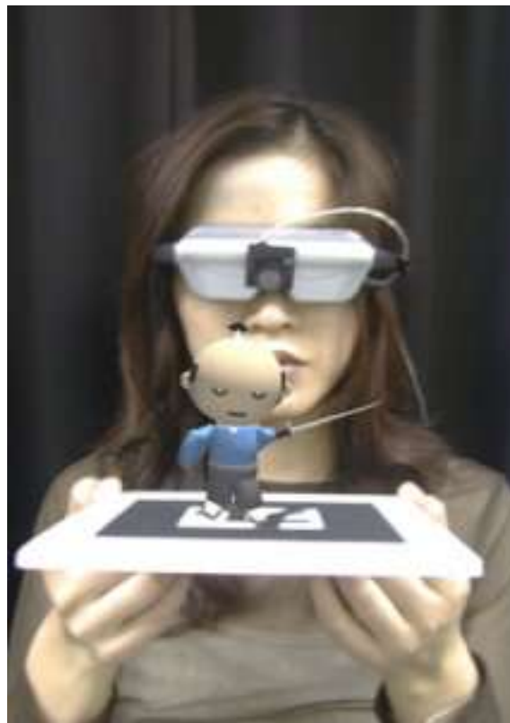
Figure 6: ARToolKit for pose tracking in 6DOF [5]
