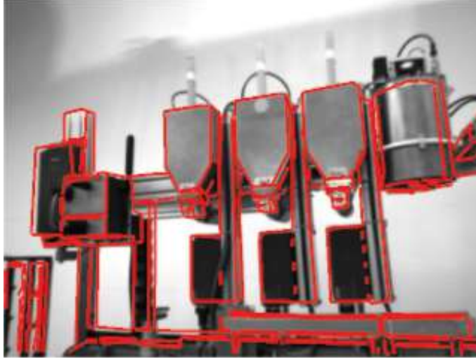
Figure 35: Model Based Tracking of industrial objects by using CAD models [43]
