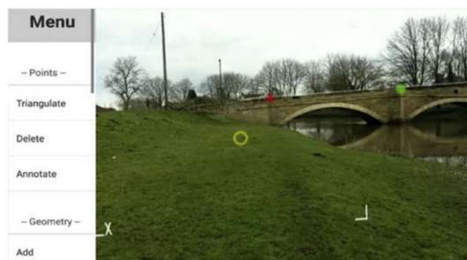
Figure 30: Browser/Authoring tool. AR tracking showing side menu, interaction annulus, and two triangulated points [11]
