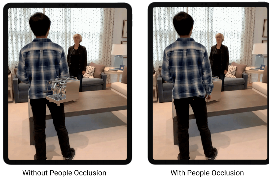
Figure 39: ARKit 3 People Occlusion, Occlusion off (left) and Occlusion On (right) [29]
