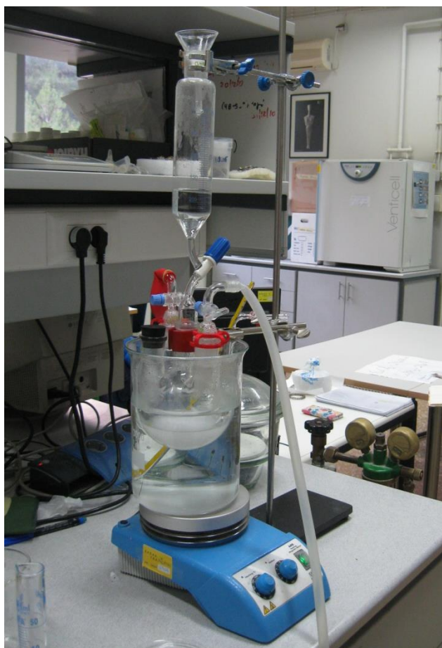
Fig. 4.4 Reactor for the synthesis of \text{Ca(OH)}_2 nanoparticles under inert conditions (He atmosphere)
