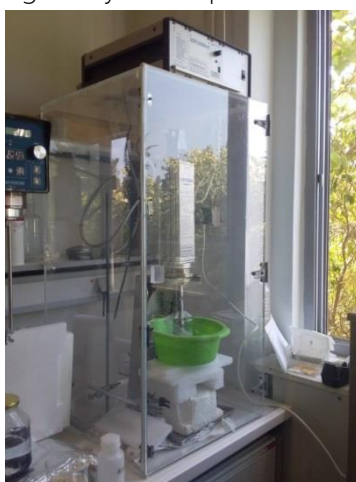
Fig. 4.3 The ultrasonic agitation unit (UIP 1000 hdTHielser) used for sonication the \text{Ca(OH)}_2 nano-dispersions.
