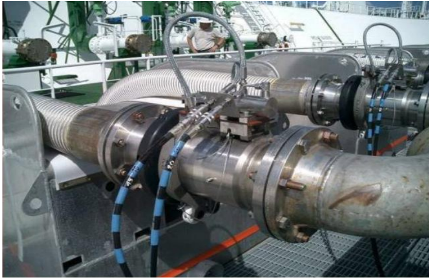
Figure 40. Emergency Release Coupling (source Excelerate Energy)
