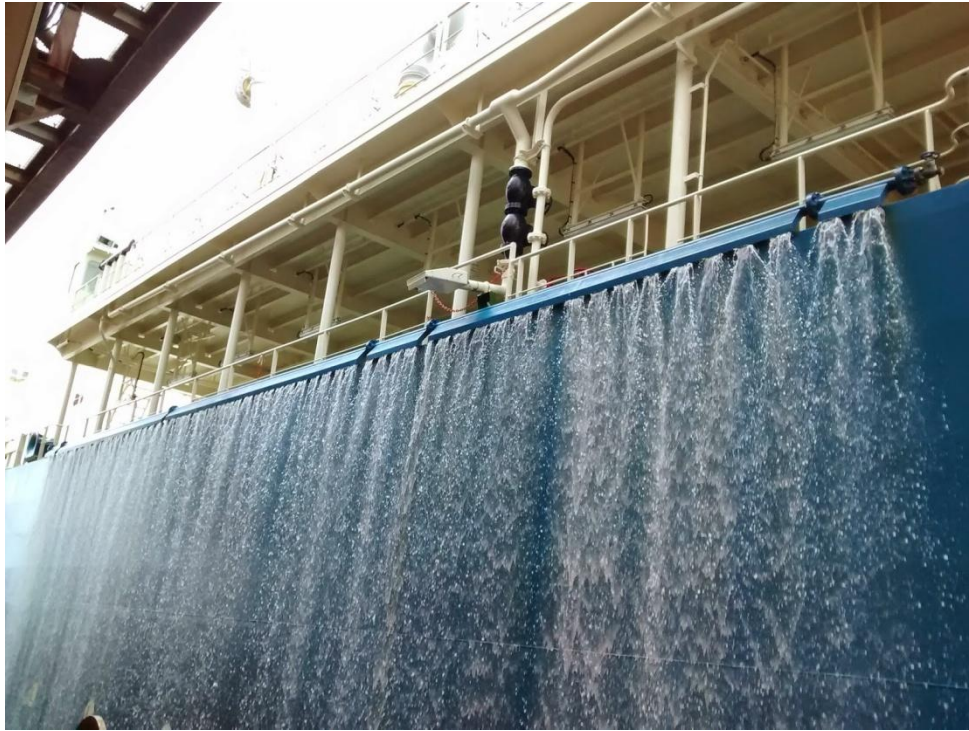
Figure 58. Water curtain utilized during LNG STS transfer to protect the ship's hull from a potential leak and subsequent embrittlement of its structure
