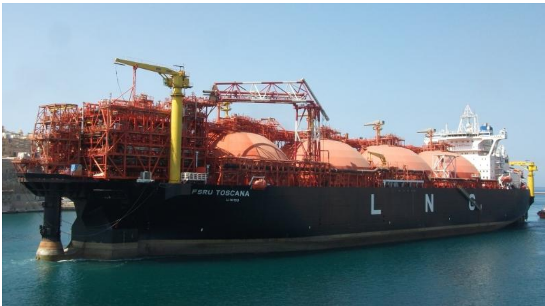
Figure 29. FRSU with Moss Type Tanks and its Regasification Facilities on the Bow of the vessel.
