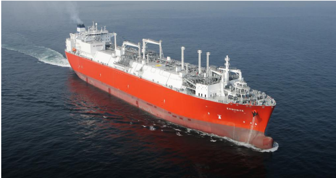
Figure 28. FSRU vessel with Membrane Tanks and its Regasification Facilities on the Deck.
