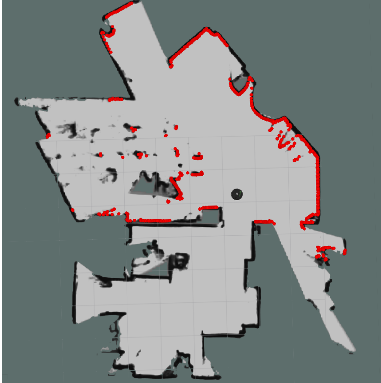
Figure 2.5: Laser Scan Example. Red Bots represent distance measurements.
