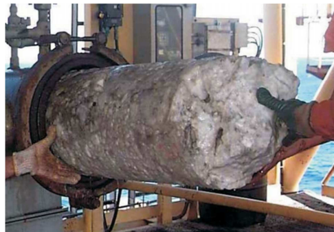
Figure 1.14: A clathrate plug recovered from an offshore gas flowline of Petrobras Company (Mao et al., 2007)
