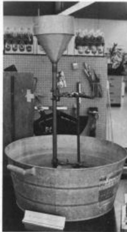
This apparatus found in the old Eaton Lab served to test abrasion effects on different products, measured by the impact of falling sand.
