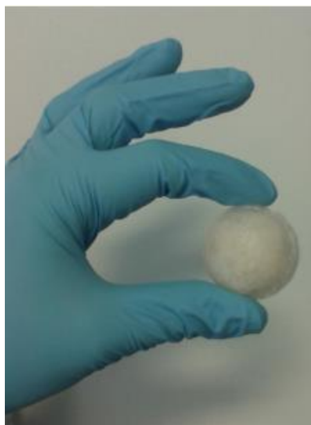
Picture 3: Sample of poly (methyl acrylate) containing 65% carbon dioxide by weight [15].
