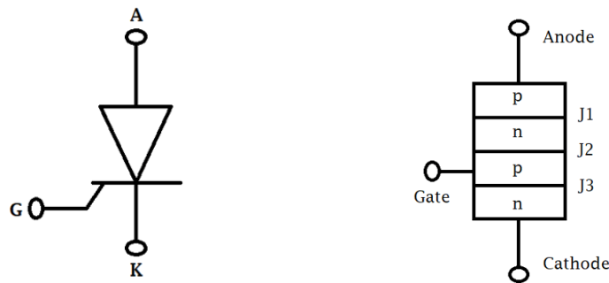
Figure 2.2: Thyristor symbol (left) and schematic diagram (right) (Khatri, 2018)
