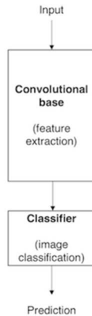
Figure 4.18 The basic architecture of CNN with the two parts Convolutional base and Classifier.[25]
