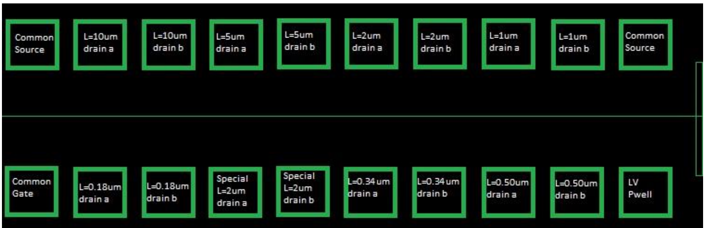
Figure 4. 3 The MOSFETs included in each die ("SPECIAL" MOSFETs were not included in the experimental process)
