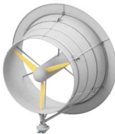
Figure 1.5: A Diffuser Augmented Wind Turbine.
