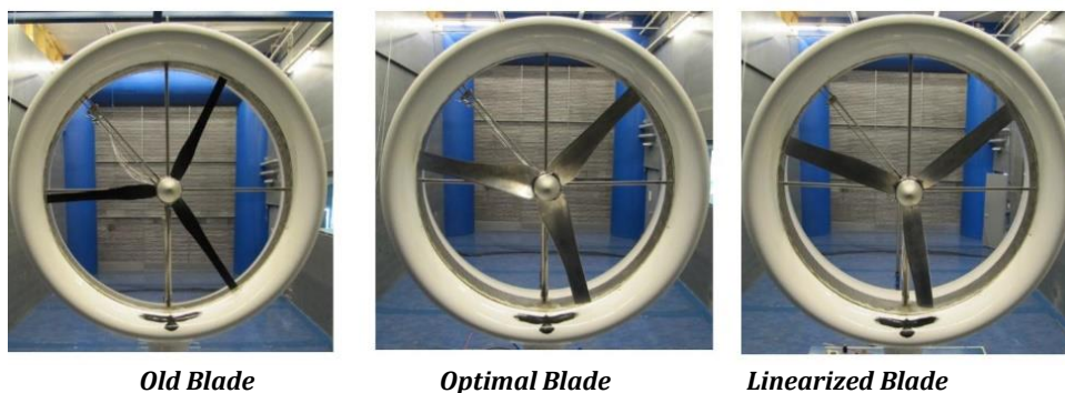
Figure 4.13: The three blade designs mounted on the diffuser of Donqi Urban Windmills [Dor11].
