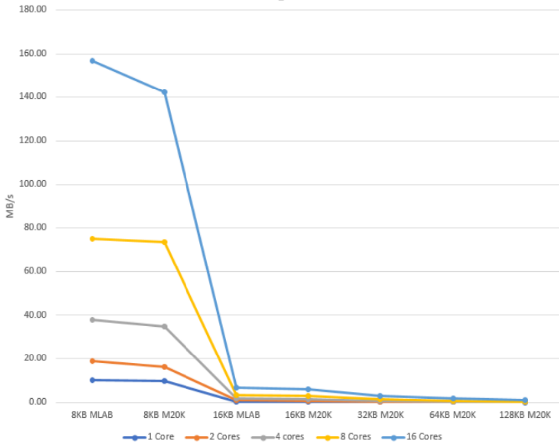
Figure 5.11: Diagram of the write bandwidth for integer matrix multiplication for different cache size/type
