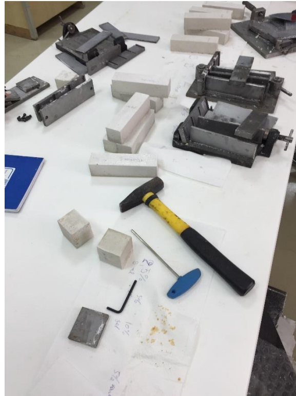
Figure 9: Demoulding of specimens after 24 hours
