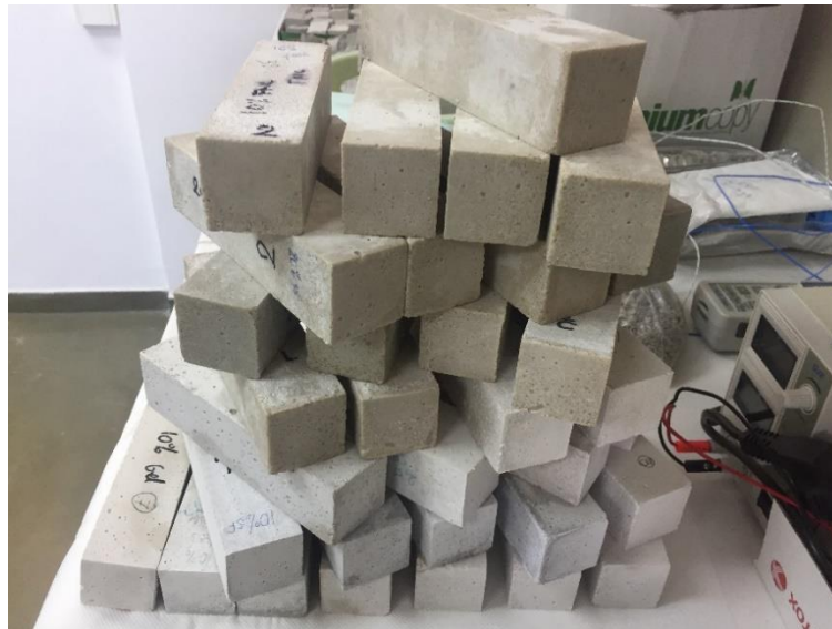
Figure 10: Specimens of mortars after 90 days of curing in a curing chamber (E139, MATEST) with stable conditions at 27-30 °C and relative humidity of 90%.
