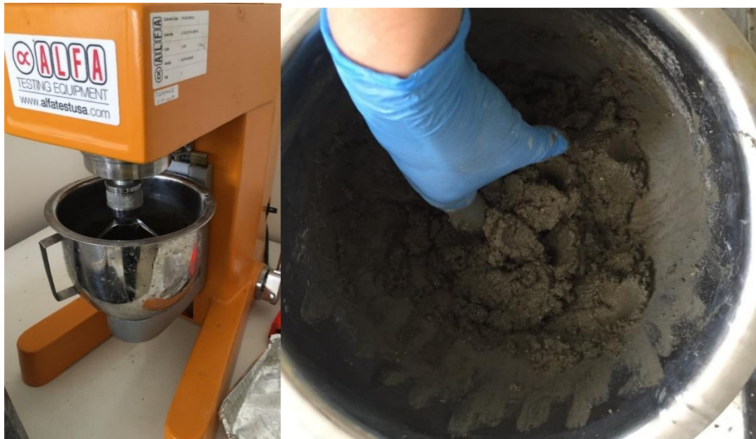
Figure 7: Preparation of cement mortars
