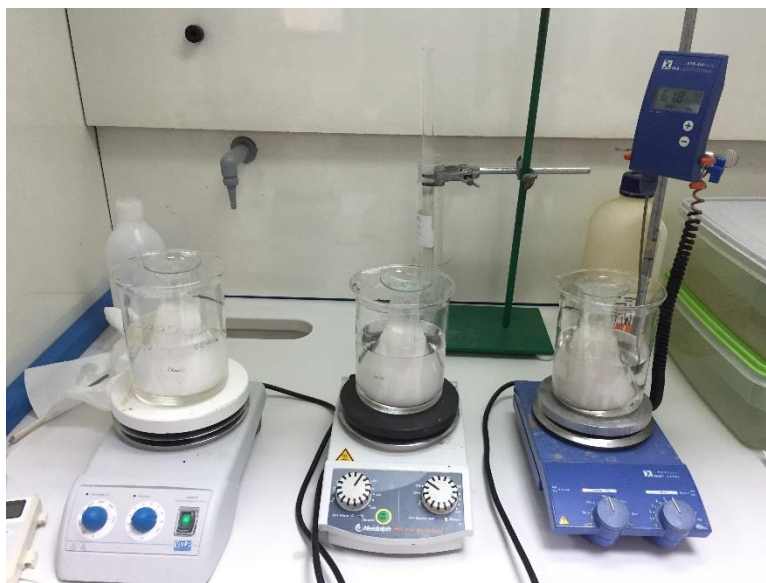
Figure 5: The apparatus of Chapelle test
