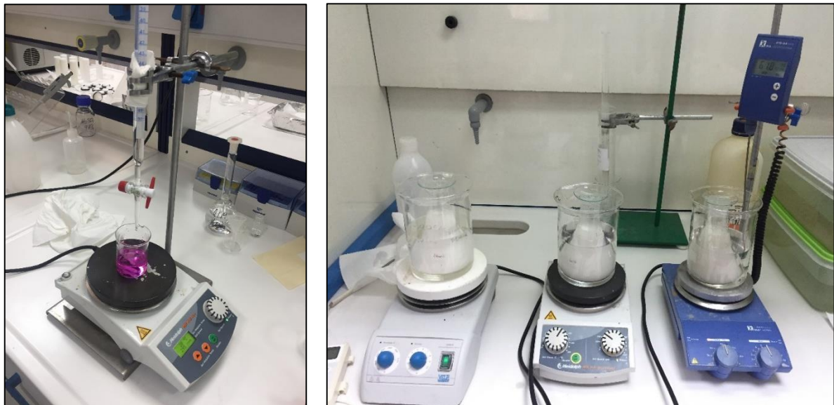
Figure 4.5: Apparatus of Chapelle test
