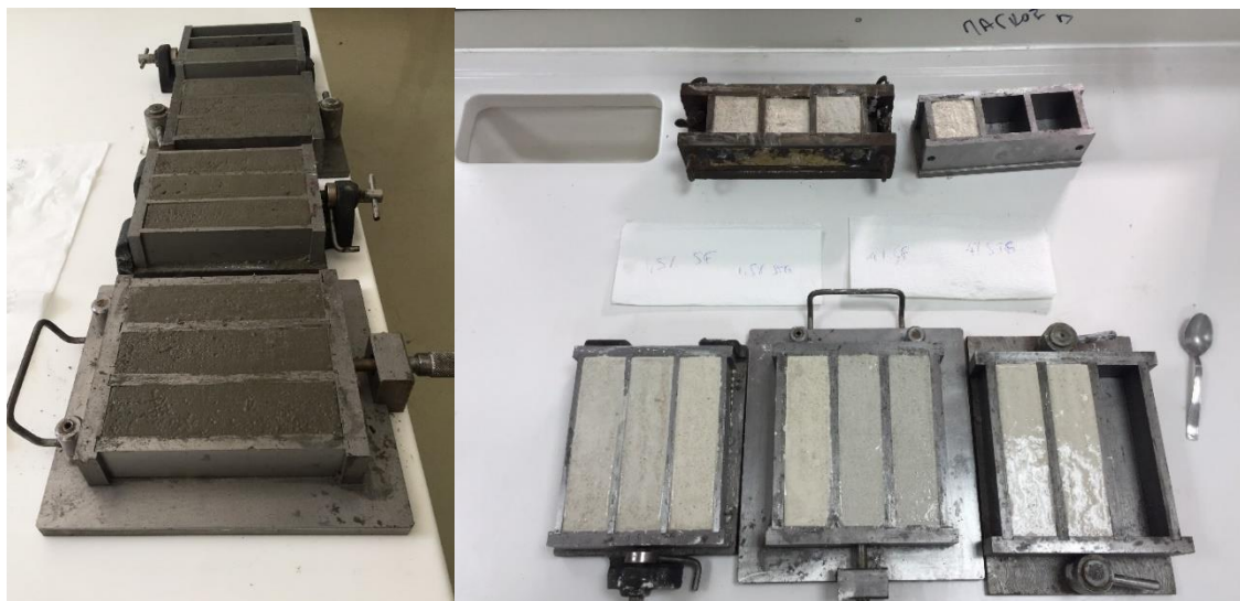
Figure 8: Casting of cement mortars into prismatic steel moulds 4 \times 4 \times 16 \text{ cm}^3
