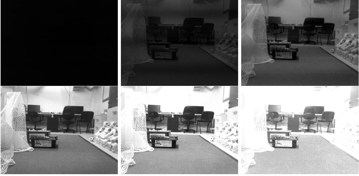
Figure 4.5: A small portion of the dataset’s images used for calibration (in grayscale), showing a static scene with increasing exposures from left to right and from top to bottom
