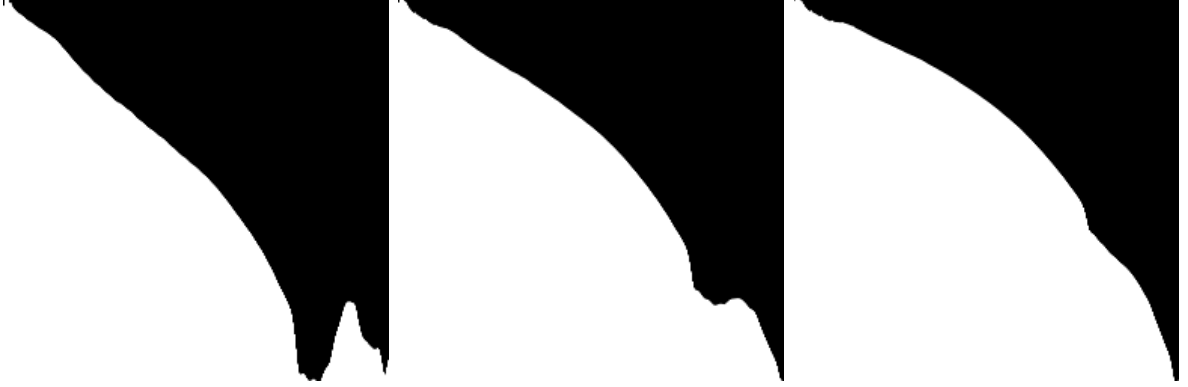
Figure 4.7: Evolution of the inverse camera response function estimation during the dataset with enabled gamma correction from left to right. In the x-axis is the pixel intensity value, and in the y-axis the irradiance
