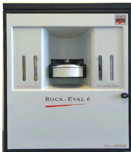
PICTURE 4.1: Rock-Eval Analysis apparatus (Laboratory of PVT and Core Analysis, Technical University of Crete).
