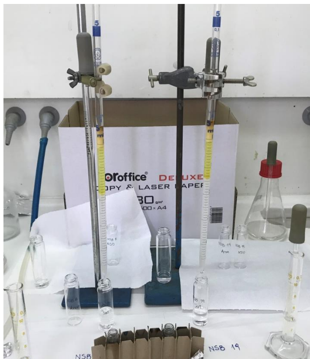
PICTURE 4.4: Column Chromatography method (Laboratory of PVT and Core Analysis).
