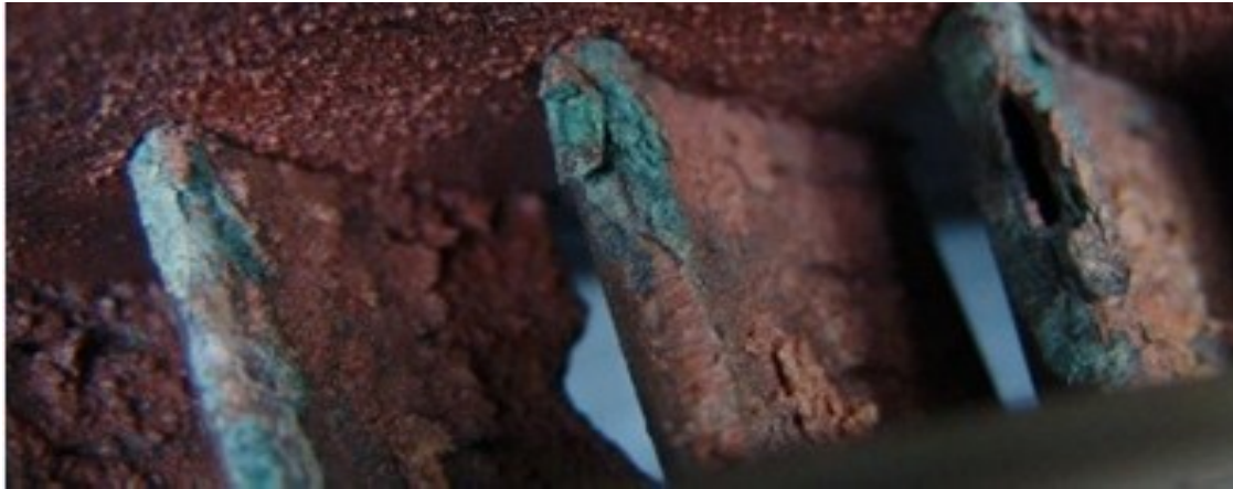
Fig. 1.3: Fouling due to sand ingestion [Szczepankowski et al., 2017].
