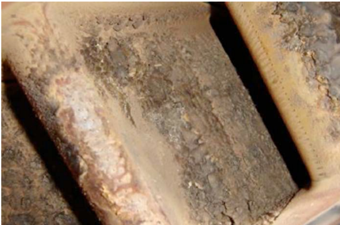
Fig. 1.2: Fouling due to deposition [Stalder, 2001].
