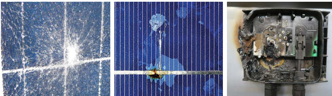
Fig. 2.1: Solar panel defects (broken glass, hot spots-burnt cells, melted junction box)
