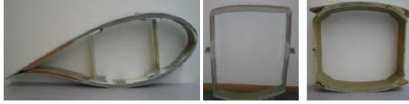
Figure 2: Different wind turbine blade designs: (2a) LM-Glasfiber design, (2b) SSP-Technology design, and (2c) Vestas design. (Mølholt, 2008)
