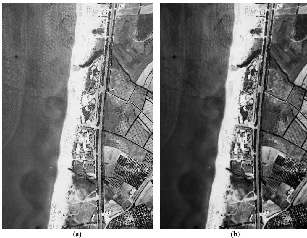
Figure 6. Automated coastline extraction from aerial imagery. (a) Initial image, (b) filtered and enhanced image.
