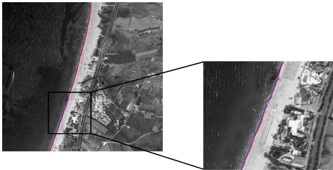
Figure 11. Estimation of the coastline and a close-up of the coastline area, applied on the second data set of aerial images. The blue line indicates the first estimation and the red line indicates the final line.
