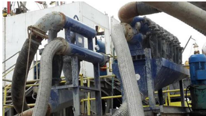
Figure 1.16. Desander and Desilter
