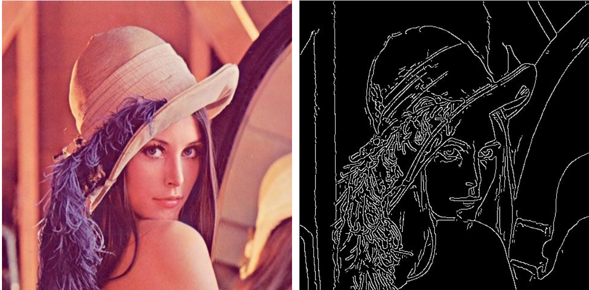
Figure 2.10: Source image (left) and Canny's output image (right).
