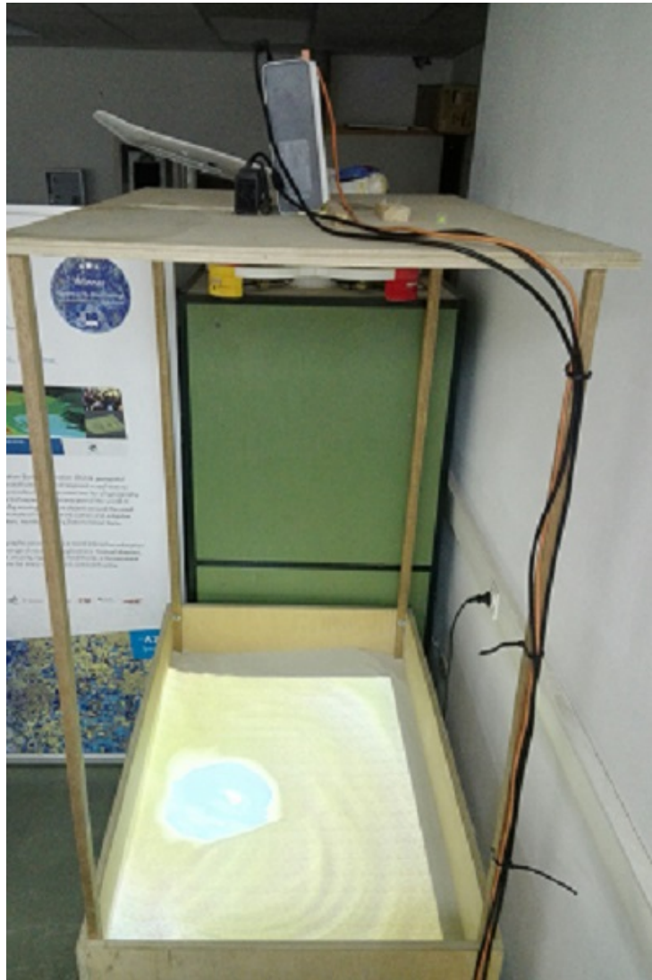
Figure 4.2: The Kinect and Projector Setup
