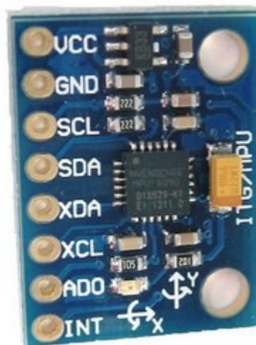
Figure 5.3 MPU-6050. Inertial Measuring Unit module
