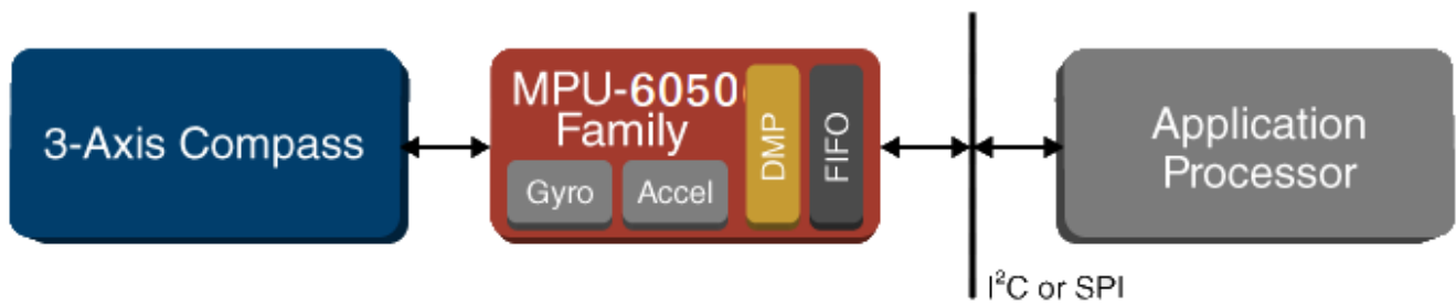
Figure 5.4 MPU-6050 Communication Level
