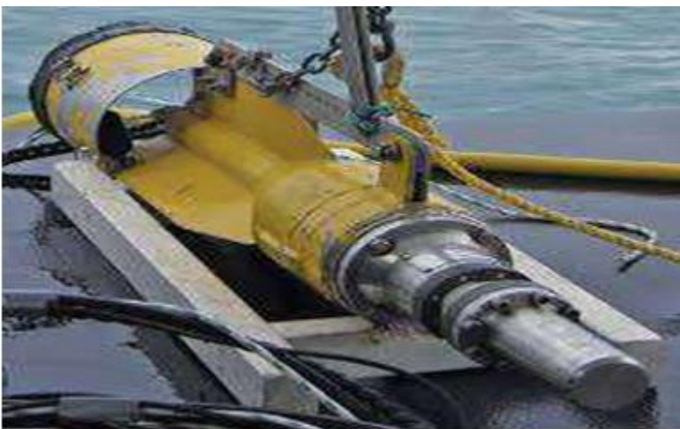
Figure 11: Bolt 600B air-gun with a 20 in3 firing chamber and bolted into a yellow tow fish (JIP).
