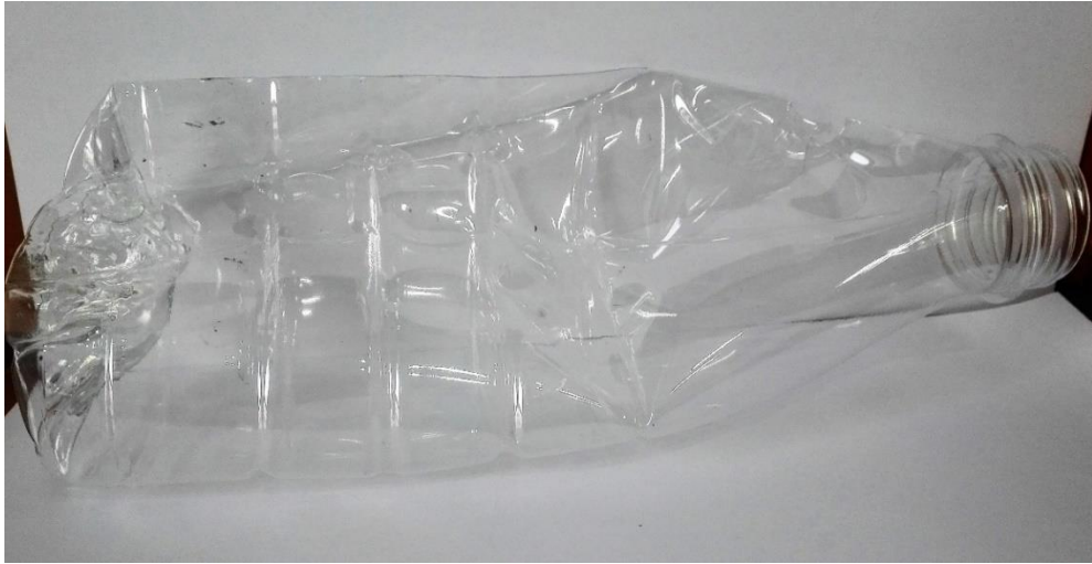
Picture 29. Damaged bottle because of bag packaging
