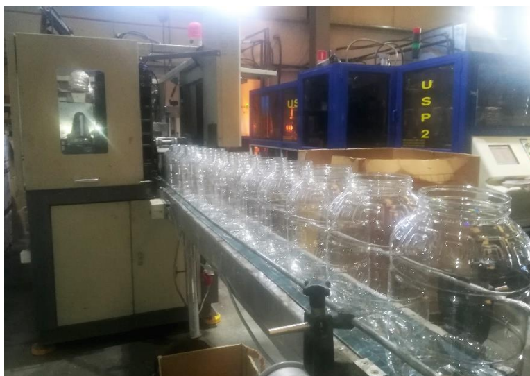
Picture 24. Conveyor belt that transfers the final product
