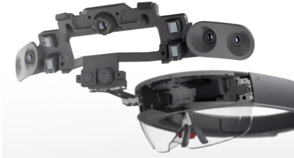
Figure 2.12. Internal sensors of the HoloLens.
