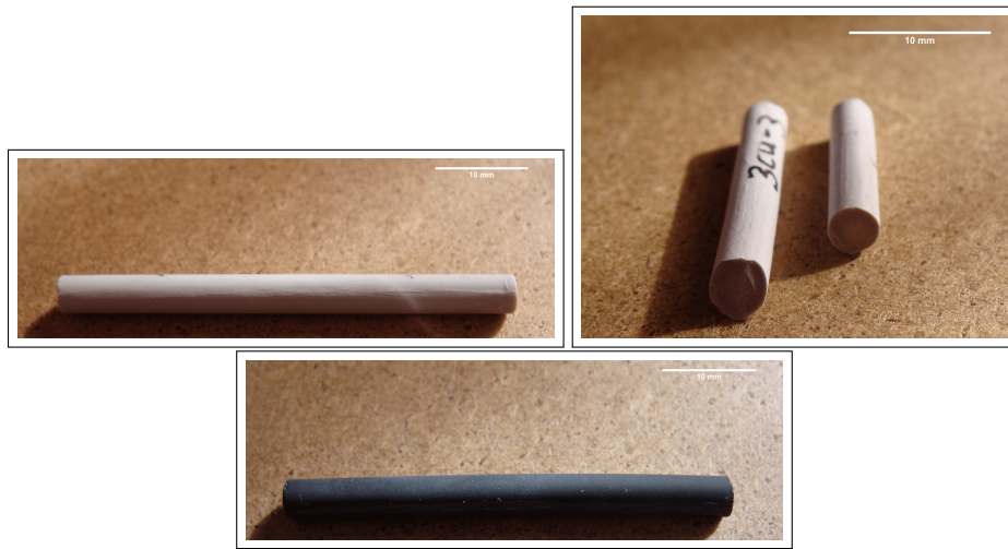
Figure 5.1: Images showing some specimens after sintering: (a) pure \text{Al}_2\text{O}_3 , (b) core-skin macro-structure for \text{Cu-Al}_2\text{O}_3 , (c) \text{W-Al}_2\text{O}_3 .
