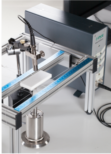
Figure 3.10: Impulse excitation technique apparatus for Young's modulus evaluation.
