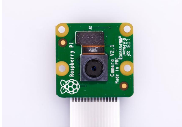
Figure 11: Raspberry Pi Camera
