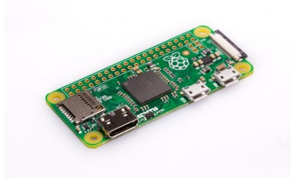
Figure 9: Raspberry Pi Zero
