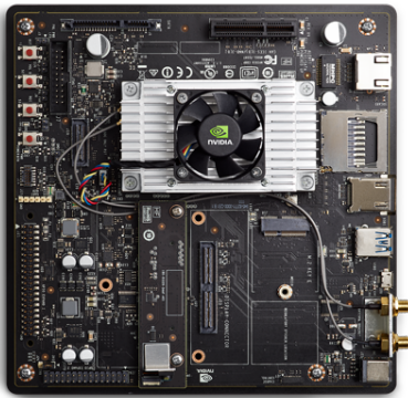
(a) Jetson TX2 Processing Unit Source: NVIDIA Corporation
