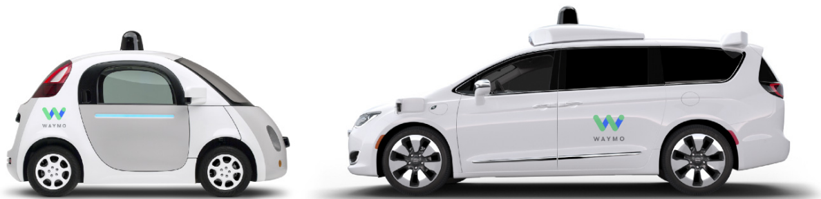
Figure 3.2: Waymo's Firefly and Chrysler Pacifica Hybrid Source: Waymo
