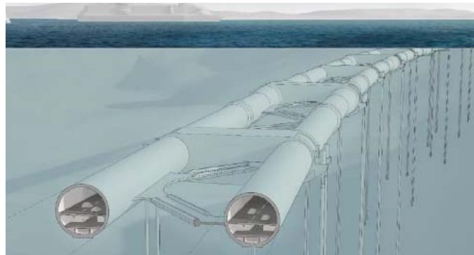
d) Submerged tunnel based on one or two tubes, with excessive buoyancy, and tethered to the seabed. Alternatively, the bridge can have less larger weight than buoyancy and be supported by pontoons in the surface.
