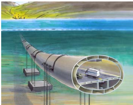
d) Submerged tunnel based on one or two tubes, with excessive buoyancy, and tethered to the seabed. Alternatively, the bridge can have less larger weight than buoyancy and be supported by pontoons in the surface.
