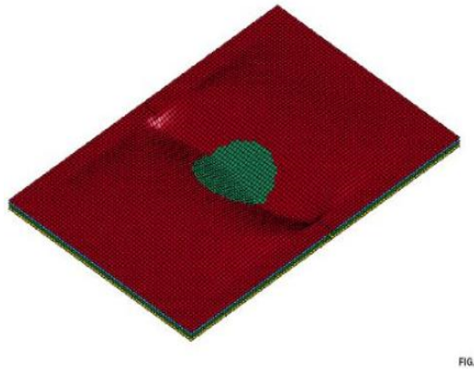
Figure 5 CAI failure mode of the numerical model
