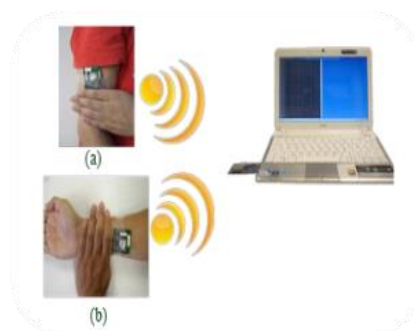
Figure 19: Sensor network consist of 2 IMUs: (a) on arm, (b) on wrist (Lee et al. 2013).
