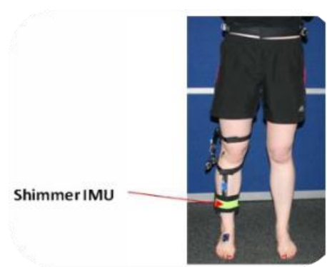
Figure 20: Single IMU placed on shin (Giggins et al. 2013).
