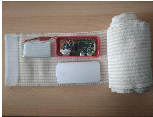
Figure 67: Resulting sensor node & Elastic bandage for stabilization on patient's knee.
