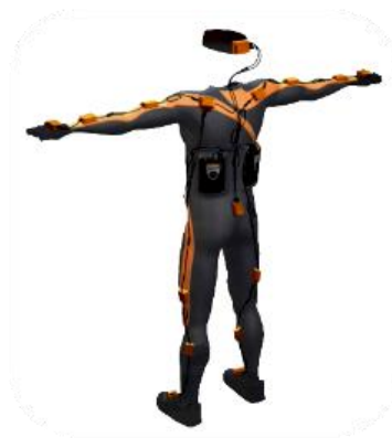
Figure 12: Xsens motion capture suit employs 17 MIMUs (Roetenberg et al. 2009).
